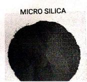
Microsilica or silica fume is an excellent admixture for concrete as it leads to better engineering properties. It reduces thermal cracking, improves durability, and increases strength. Silica fume concrete has a number of construction applications.
